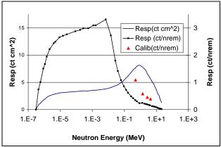
Figure A-2. Fluence and dose response vs. energy for PMS neutron detector (Liu et al. 1991) [11]
