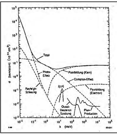
Figure 2-2. Photon cross sections for copper.
