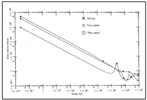
Figure A-1. Cross section versus neutron energy for some reactions of interest in neutron detection (Knoll 1989, Figure 14-1)
