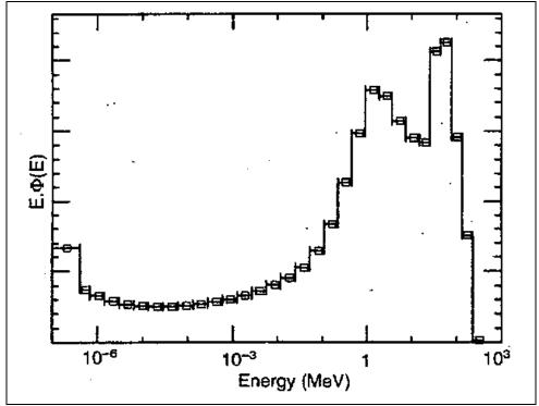
Figure 2-5. Neutron spectrum from 46.6-GeV electrons through iron and concrete (Vylet et al. 1997).
