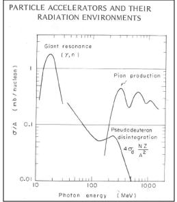
Figure A-3. Neutron Production from Electromagnetic Cascade
