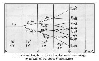
Figure A-2. Electromagnetic Cascade
