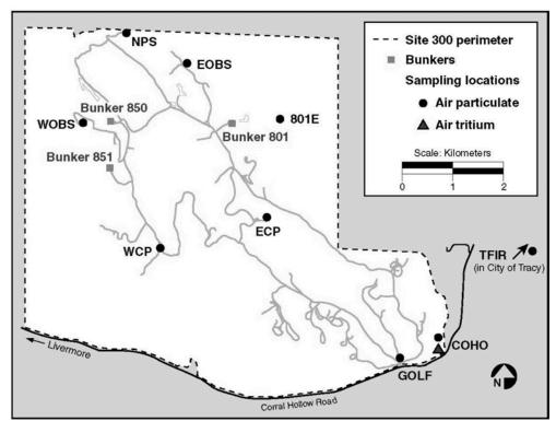
Figure 2-3. Site 300 map with bunkers and air-sampling stations (Gallegos et al. 2002, Figure 5-3).
