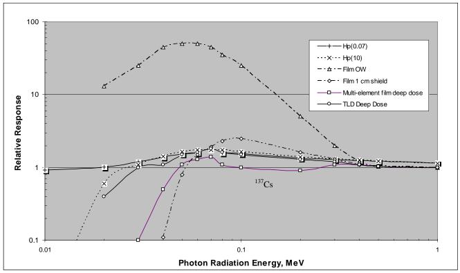
Figure 6-1. Typical two-element, multi-element film and TL dosimeter photon response compared to Hp(0.07) and Hp(10).
