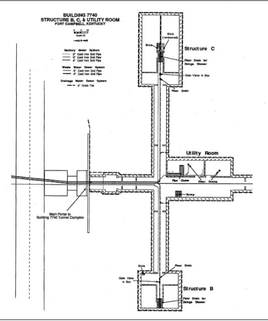
Figure 2-4. Plan view of the B and C Structures in the tunnel complex.
