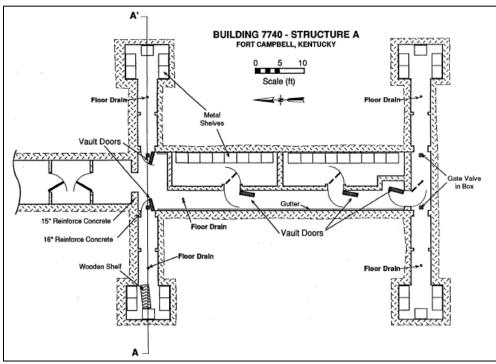
Figure 2-2. Plan view of the A Structure.
