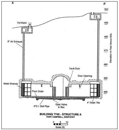
Figure 2-3. Cross-sectional view of the A Structure.
