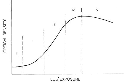
Figure 1. Characteristic Response Curve (H & D) for a Photographic Emulsion Exposed to Ionizing Radiation (Source: NRC 1989)
