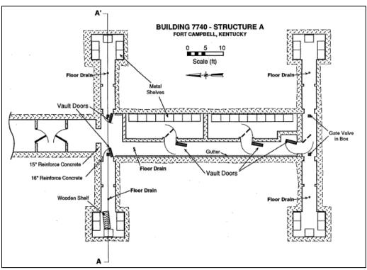
Figure 2-2. Plan view of the A Structure (Last, Gilmore, and Bronson 1998).
