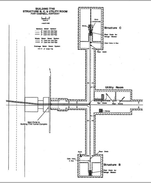
Figure 2-4. Plan view of the B and C Structures in the tunnel complex (Last, Gilmore, and Bronson 1998).
