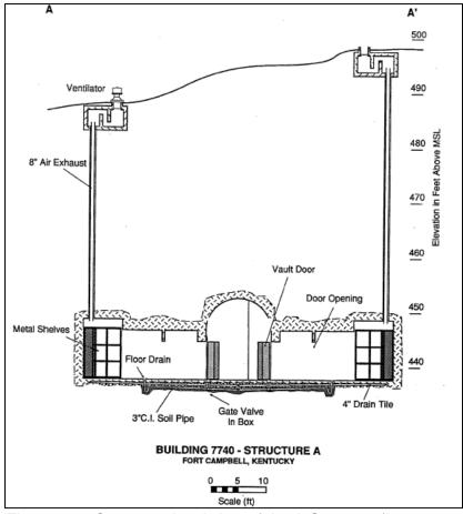
Figure 2-3. Cross-sectional view of the A Structure (Last, Gilmore, and Bronson 1998).
