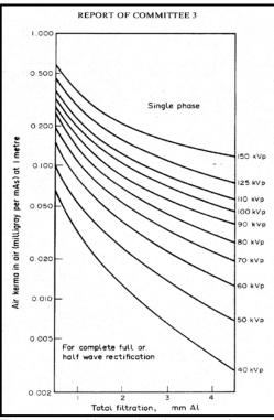
Figure 3-1. Kerma in air at 1 m from X-ray source as a function of total filtration for various values of tube potential (ICRP 1982).
